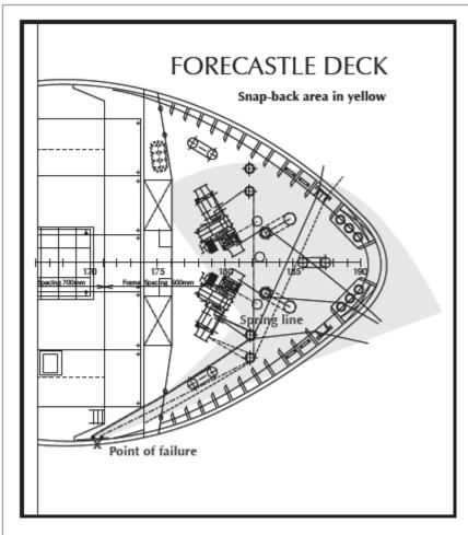
The diagram shows the potential area of danger (snap-back zone) when the spring line parts at the spring line fairlead. The snap-back zone would be increased if both pedestal fairleads were used. (Swedish Accident investigation Authority Report S-95/11 Morraborg)
